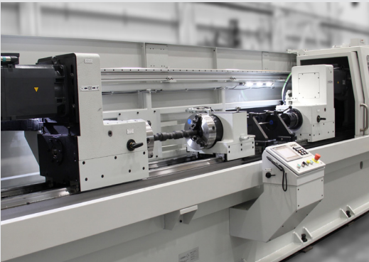
Rolling guards with full access to workpiece and tooling
